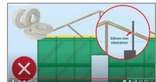
Minimum 50mm clearance of insulation/sarking from hot flues
