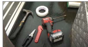
Typical tools for sarking tied roofs
